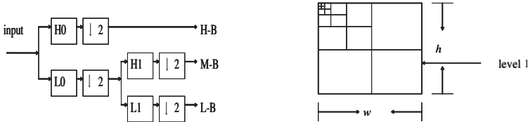
Fig. 1. 1-D DWT Diagram and 16 Subbands in a 5-level 2-D DWT
